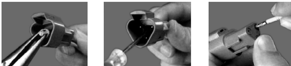
Figure 7-13. DT/DTP Contact Removal
