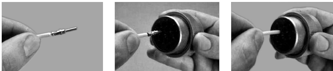
Figure 7-14. HD/HDP Contact Installation
